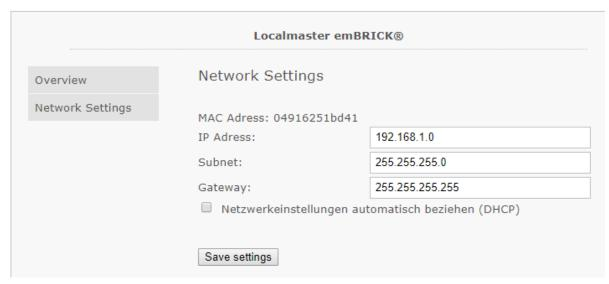
In the Network settings you will see the used MAC-address and you can change the IP settings of your coupling brick. Before doing this, set the DIP-switches to "0001". If you don't set them to the position "0001", the IP Adress of the DIP-switch is set. You can reboot the system by clicking on the onboard reset button.
